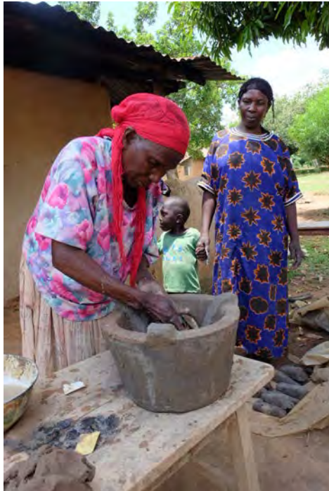
A woman in Siaya makes an energy efficient stove that she will sell to community members.
